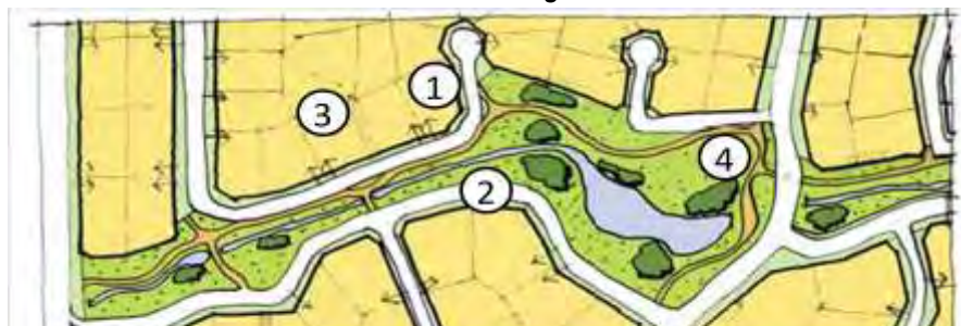
Figure 2: Concept illustrating the use of roading along the gully to make the gully system more legible and reduced densities around the gullies to protect the natural and ecological environment.
