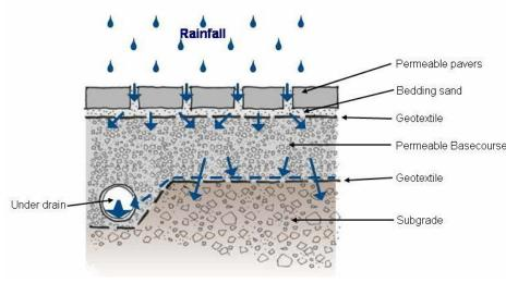
Figure 1: Typical layers in permeable pavement
