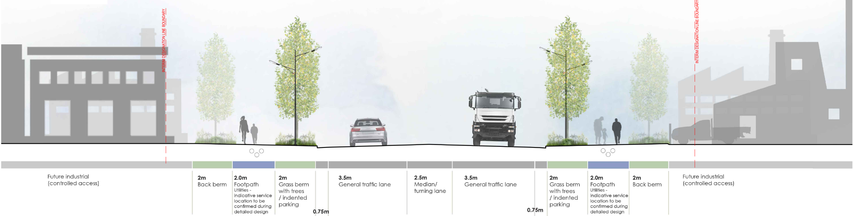
TYPICAL SECTION 6 - COLLECTOR ROAD, ARTHUR PORTER DRIVE (3102.2) WIDTH 23.0m SCALE N.T.S
