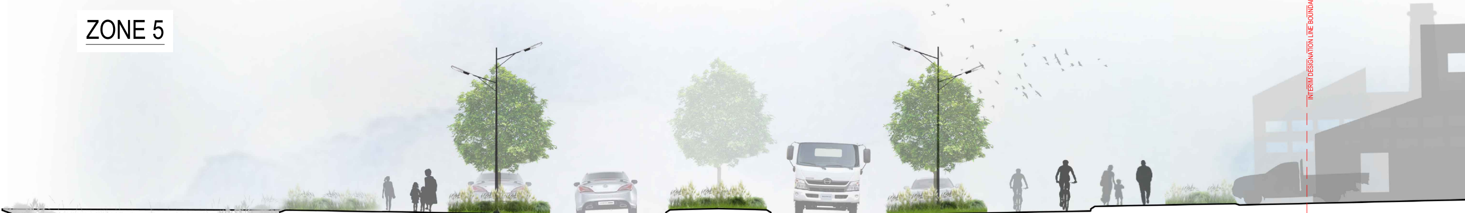
TYPICAL SECTION 4 - COLLECTOR ROAD, CHALMERS ROAD EXTENSION (3122.2) WIDTH 23.8m SCALE N.T.S
