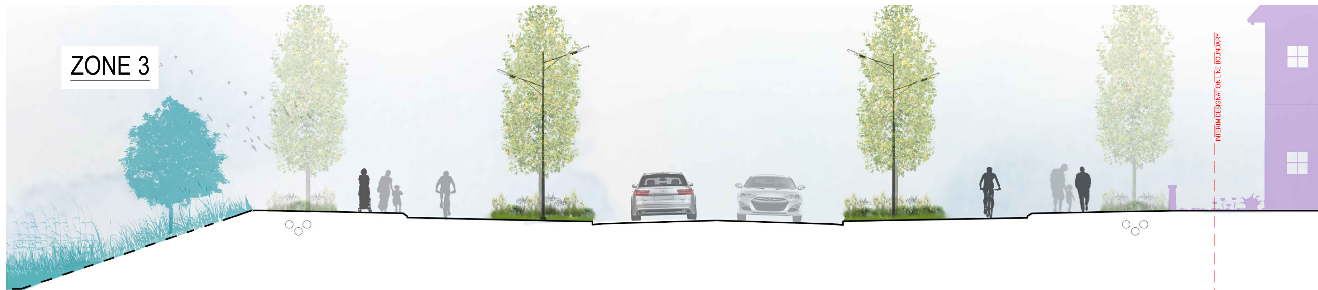
TYPICAL SECTION 2 - MINOR ARTERIAL, TE KOWHAI ROAD WEST EXTENSION (3101.3) OPTION A, WIDTH 29.4m SCALE N.T.S
