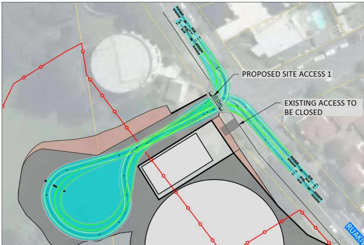
Figure No: 14 – 19.45m HPMV tracking analysis at Site Access 1 and onsite manoeuvring
