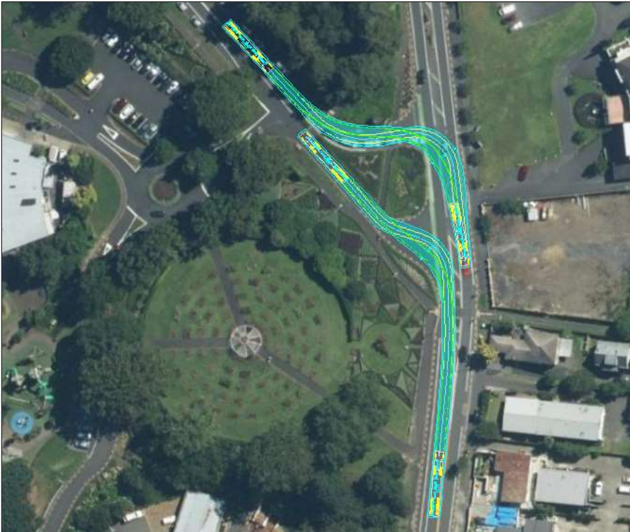
Figure No: 12. 19.45m truck turning at Pembroke Road / Ruakiwi Road intersections
