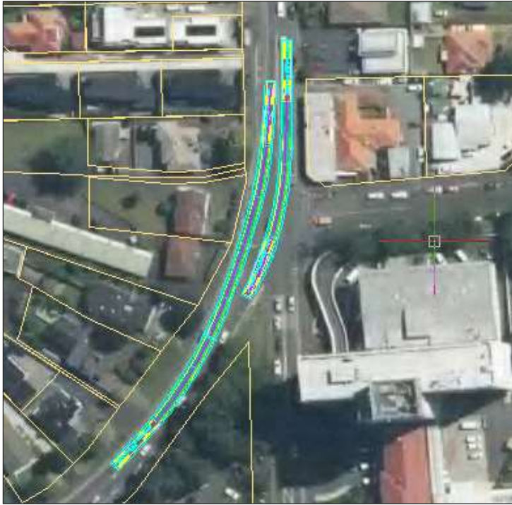
Figure No: 10. 19.45m truck passing at Pembroke Street / Selwyn Road Intersection
