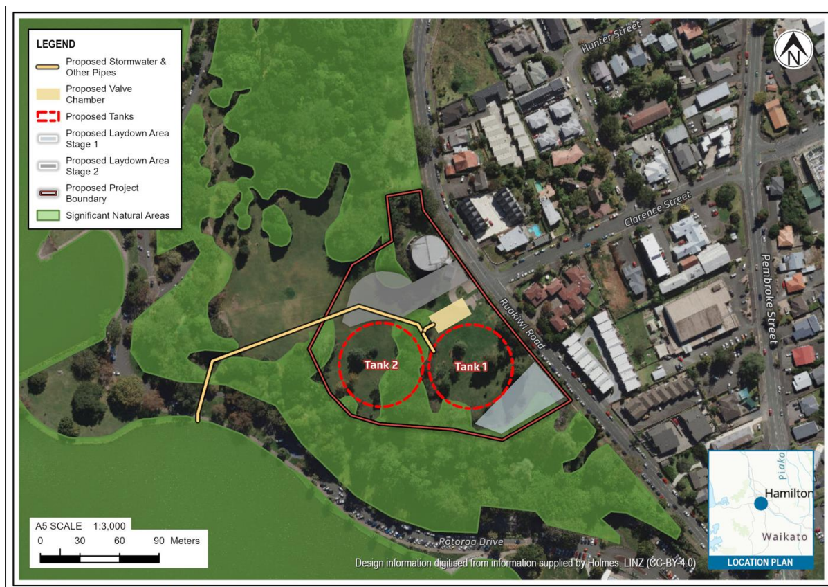
Figure 1.1: Project location with proposed water reservoirs, pump valve chamber, proposed stormwater pipes and Significant Natural Areas.
