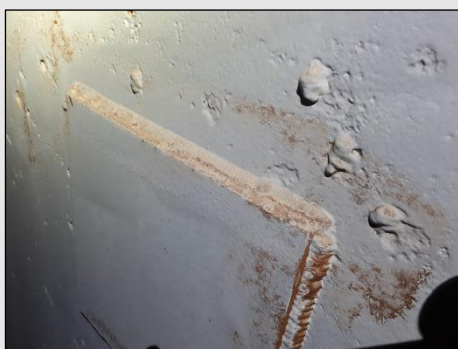
Figure 3 - Patch repair and ugly weld filling, rough edges heavy pitting along bottom strake
