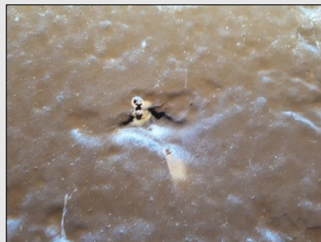
Figure 2 - Pitting corrosion at 6 o'clock closeup
