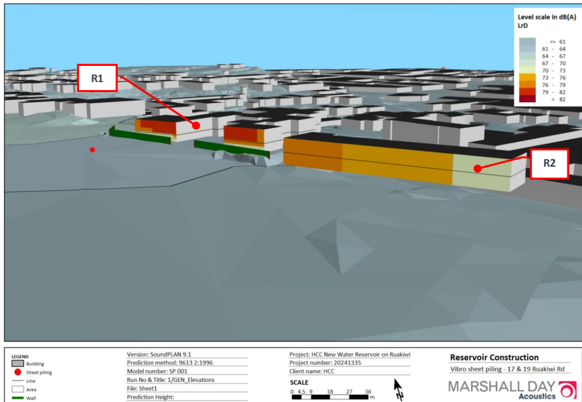
Figure 4: Vibro sheet piling noise received by 17 & 19 Ruakiwi Road
