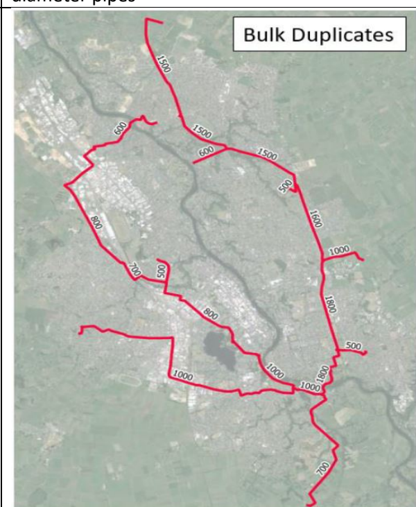
Figure 4. – Bulk Ring Main, duplicate pipelines needed to service proposed (Citywide) NPS Densities
