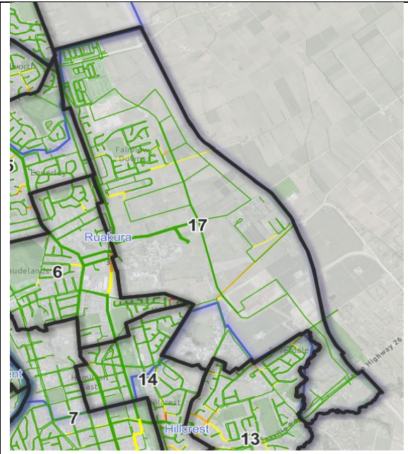
Figure 2. – 2031 Headloss 40mm and above diameter pipes
