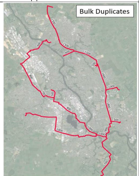
Figure 4. – Bulk Ring Main, duplicate pipelines needed to service proposed (Citywide) NPS Densities
