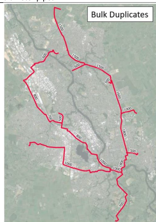
Figure 4. – Bulk Ring Main, duplicate pipelines needed to service proposed (Citywide) NPS Densities
