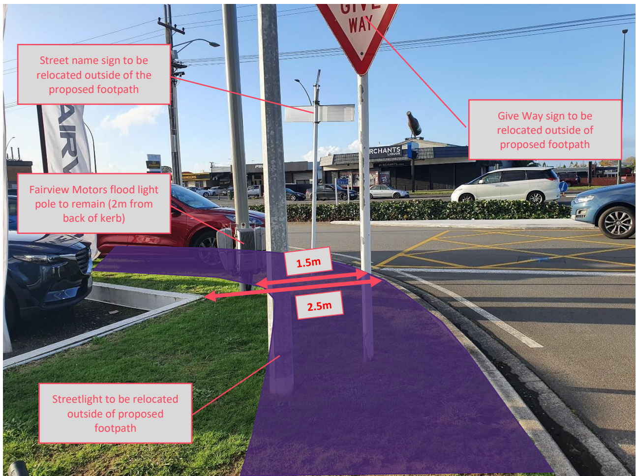
Figure 35: Signs and Light Poles to be Relocated to Accommodate Footpath
