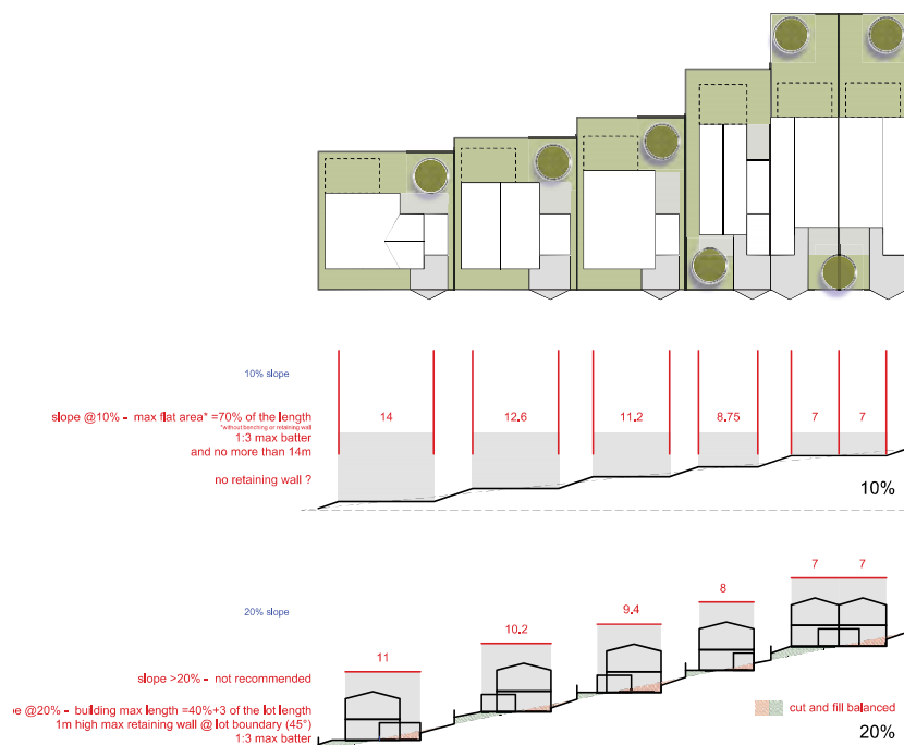
Figure 15: On sloping ground, lot orientation and size should be considered to reduce the extent of retaining required (Mensagh Graham - Peacocke Landscape assessment - 2021) .
