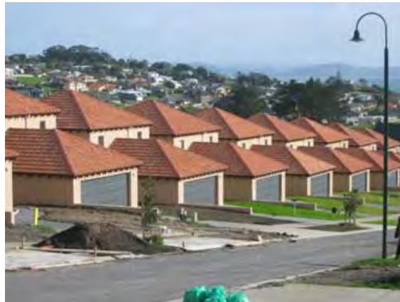
Figure 1.4.2e: Garage doors forward of the front face of buildings should be discouraged
