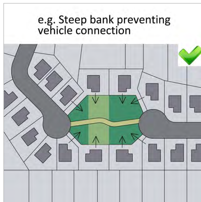
Figure 1.4.1o: Where vehicle connections cannot be made culs-de-sac should include, where appropriate, pedestrian and cycle links
