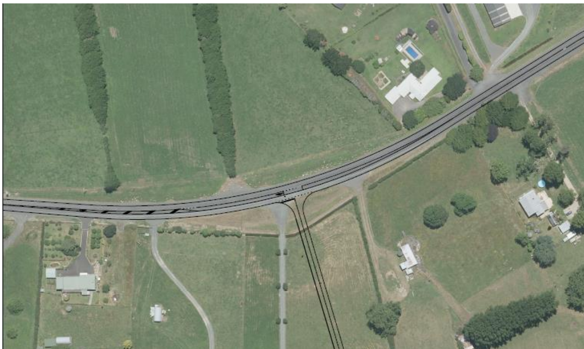
Figure 6-8: Collector 1/ SH39 intersection (give-way) – indicative layout
