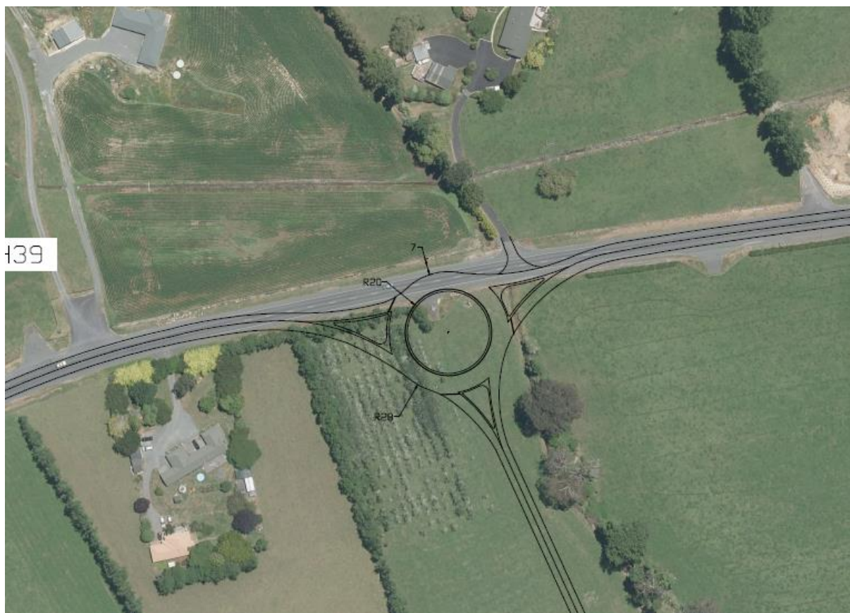
Figure 6-9: Collector 2/ SH39 intersection (roundabout) – indicative layout
