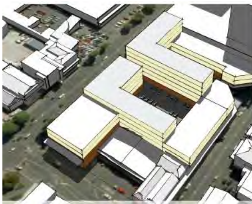
Figure 1.4.5q: Future development preference – 3D model showing potential built form, with through-site links, internal courtyards and veranda cover
