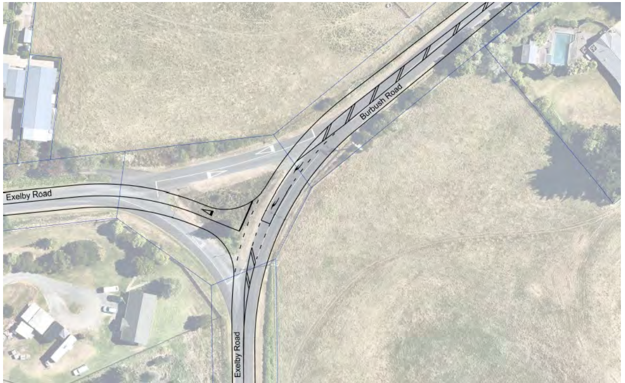
Figure 13: Exelby Road / Burbush Road intersection (upgrade)
