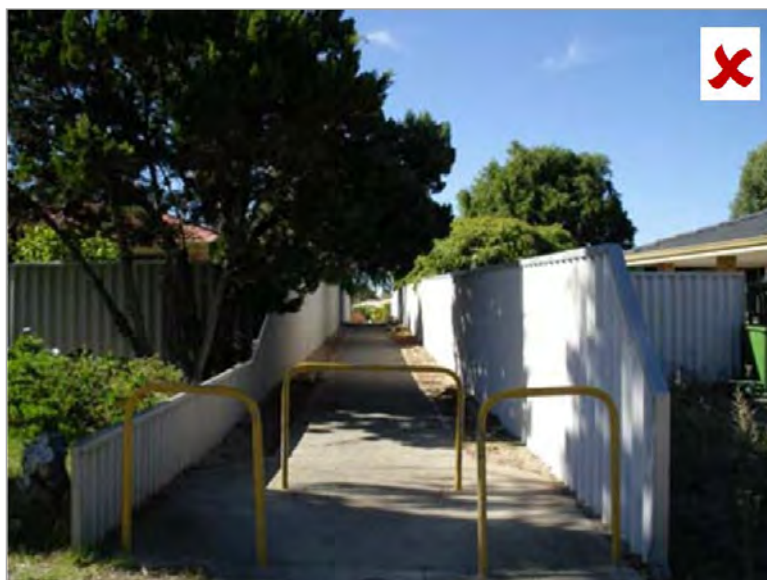
Figure 1.4.1f: Poorly designed interface with pedestrian accessway. High, visually impermeable fences, poor lighting and landscaping prevents passive surveillance
