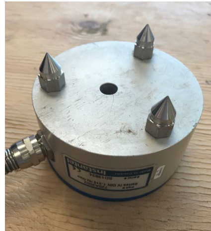
Figure 6: Transducer set up with carpet spikes.
