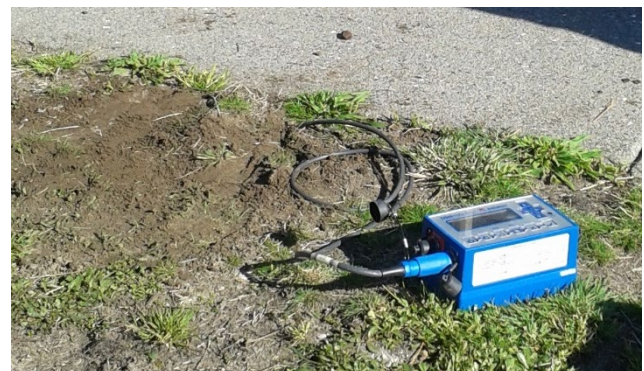
Figure 10: Vibration monitoring device set up with the transducer buried in the ground.
