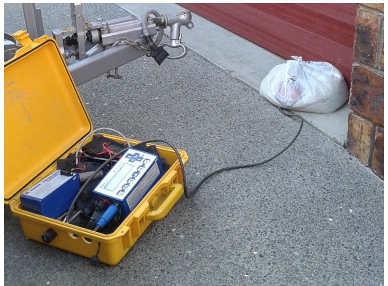
Figure 7: Vibration monitoring underway on the concrete slab foundations of a garage. The transducer is placed directly on the concrete (i.e. no spikes are used) and the transducer is weighed down with a 7kg sandbag.
