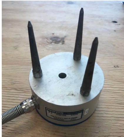
Figure 5: Transducer set up with ground spikes.
