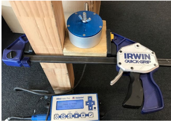
Figure 8: Monitoring annoyance vibration. Monitoring device set up next to an office desk using a piece of wood clamped to an internal pile. A bolt with wing nut is used to fix the transducer to the block of wood.
