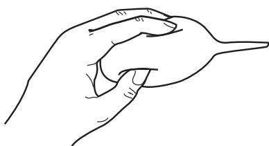
1. Squeeze the air out of the bulb.
