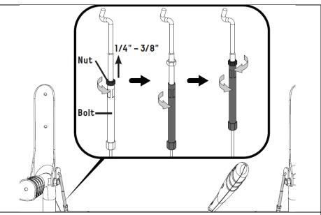
While operating the snowblower, if the auger control lever is too loose, tighten the nut counter-clockwise while at the same time rotating the bolt upward to reach the position of the nut.
