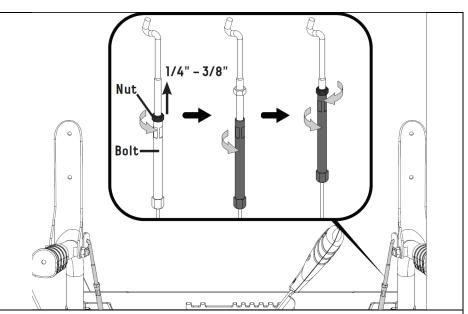
While operating the snowblower, if the drive control lever is too loose, tighten the nut counter-clockwise while at the same time rotating the bolt upward to reach the position of the nut.
