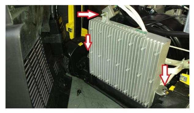
3. Begin disconnecting the control unit's wire harnesses. You can now discard the old module and install replacement module. Reverse previous steps to complete service.
