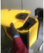
3. Remove (4) corner panels. 4. Unscrew the screws to remove the right cover. Repeat for the left cover. 5. Unscrew the (3) bolts that hold the fuel tank.
