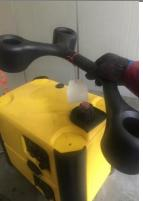
2. Unscrew the fuel tank cap and remove the upper cover.
