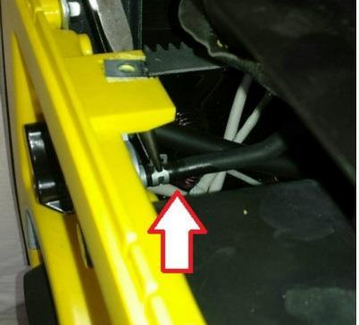
4. With the hoses disconnected, you can remove the 7mm fuel tank bolts and set the existing fuel tank aside. Replace with new fuel tank and reverse these steps to complete install.
