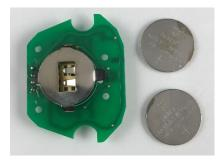
5. Replace old batteries with two (2) new **CR2016** batteries with the batteries stacked on top of one another with the positive (+) sides facing up.
