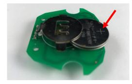
6. Using a small straight blade screwdriver, bend the retaining tab back down.
