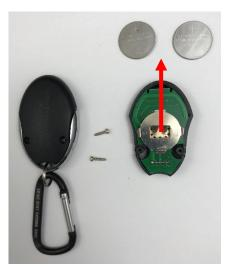
3. Replace old batteries with two (2) new **CR2016** batteries with the batteries stacked on top of one another with the positive (+) sides facing up.
