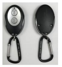
1. Remove two (2) screws from the back of the remote fob using a philips screwdriver. Separate back cover from front.
