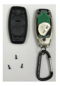
2. Use fingernail or flat blade screwdriver in black recessed area to pull batteries out of holder.
