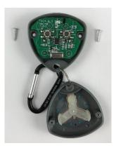
8. Place the back cover over the front and secure together with screws removed from Step 1.
