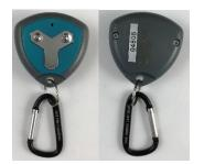
1. Remove two (2) screws from the back of the remote fob using a philips screwdriver. Separate back cover from front.
