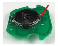
7. Insert the printed circuit board back into the back of the remote housing with the batteries facing down.
