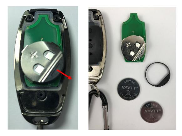
3. Replace old batteries with two (2) new **CR2016** batteries with the batteries stacked on top of one another with the positive (+) sides facing up.
