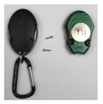
2. Push the batteries out from underneath the holder using the philips screwdriver. Note the orientation of the batteries as they come out.
