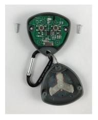
2. Remove the green printed circuit board from the remote housing.
