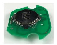
3. Using a small straight blade screwdriver, bend the retaining tab up past the top of the battery holder.
