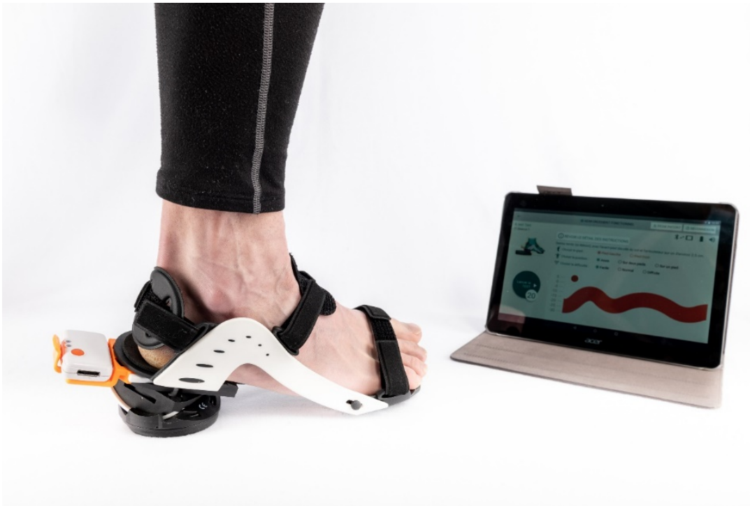
Figure 1. The ankle destabilization device used for proprioception and evtor muscle assessment (participant position and hindfoot platform).
