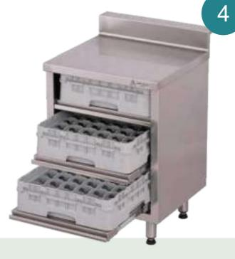
• COFFEE MACHINES FURNITURE Construction made of AISI 304 #4 finish stainless steel, with central divider, open compartment, coffee collection hopper and bottom legs with adjustable feet - Normal drawer + coffee hopper - Complete with stainless steel top with splashback
