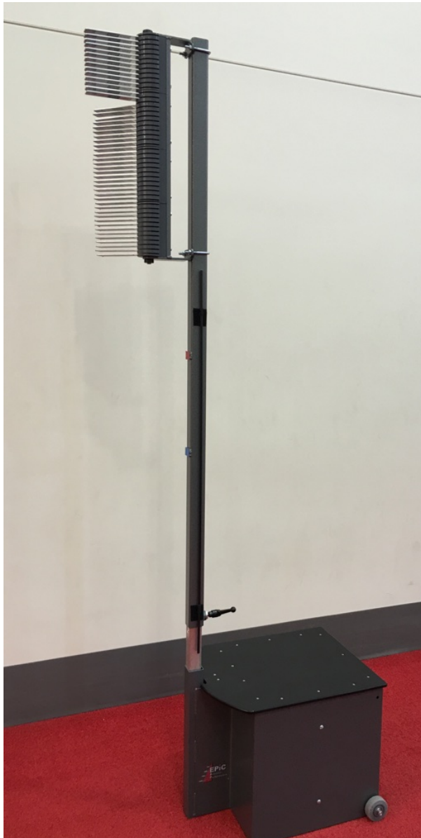
(Fig. 6) The Vertec replaced the yardstick but athletes had to have their reach subtracted from their jump to calculate the jump. In 2016 the Husker strength staff assisted in the design of the current Jump Station used by the Huskers.
