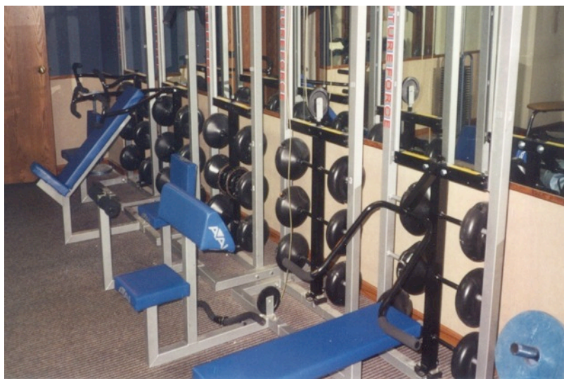
(Fig 39) The Future Force plates could be filled with water or sand. The user had a choice of 0 to 6 weights. The weights could not fall on the user or pinch their fingers.
