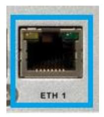
On the front panel, normally the green LED is solid with a blink every three seconds. The red LED will illuminate and blink during booting of the unit, but once the unit has booted if the red LED stays on or is blinking, it indicates a problem locking onto the audio stream and/or with the unit configuration.
