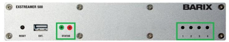
Do not use the reset button on the front panel of the receiver, as this could delete all configuration from the unit and require you to send it back to the Huskers Radio Network for reconfiguration. If you think the unit needs power cycled, unplug the power cube from the AC power outlet for about 30 seconds, then plug the power brick back in.
