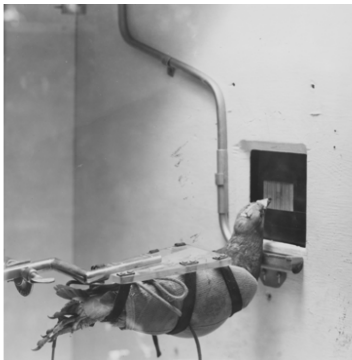
The pigeon-guided missile experiment by B.F. Skinner, commonly known as Project Pigeon , later renamed Project Orcon , for "organic control" (1944–1948). Courtesy of the B.F. Skinner Foundation.
