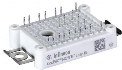
Figure 2-4: Half bridge. Picture from [9].
