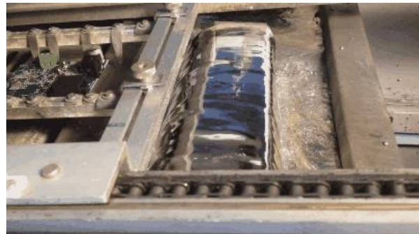
Figure 3-3: Wave soldering. Picture from [25].
