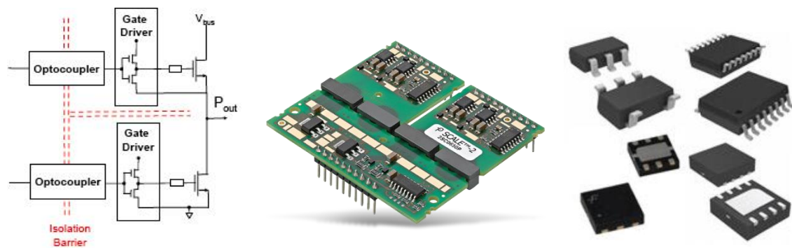
Figure 2-6: Left: Gate driver schematic [14]. Middle: Example of gate driver card [15]. Right: Example of gate driver s Picture from [16].
