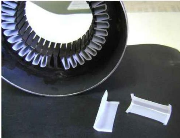
Figure 47 Slots insulation (Carnevale, 2020)
