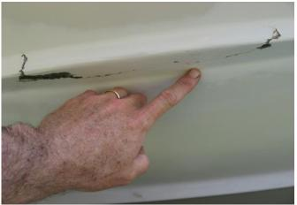
• Examine the Hull's for problem areas. This will be seen by a discoloration in the Gel-Coat. If you believe the hull was repaired, inquire about the matter. Ensure the repair was done right.
