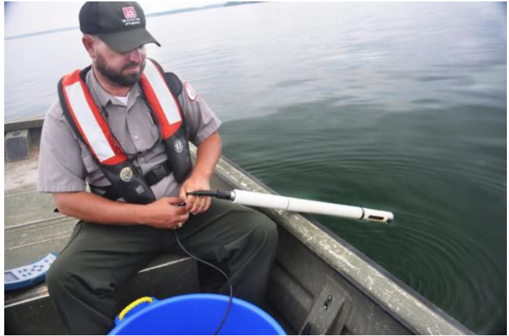
Natural Resource Specialist Jess Fleming takes water quality measurements in Lake Hartwell on the Georgia-South Carolina state line. The Corps of Engineers shares water temperature and dissolved oxygen data with the Georgia Department of Natural Resources in an effort to learn more about fish habitat and survivability in the reservoir.
