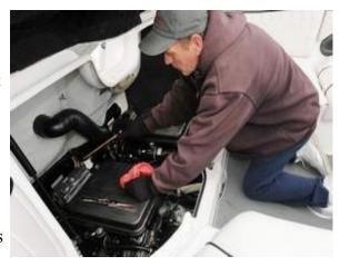
**Fourth**, the boat's gas tank should have been full so no moisture had a chance to form. Make sure that the fuel filter has been changed and its lines were not cracked. It's not uncommon to find these lines cracked from the winter temperatures.
