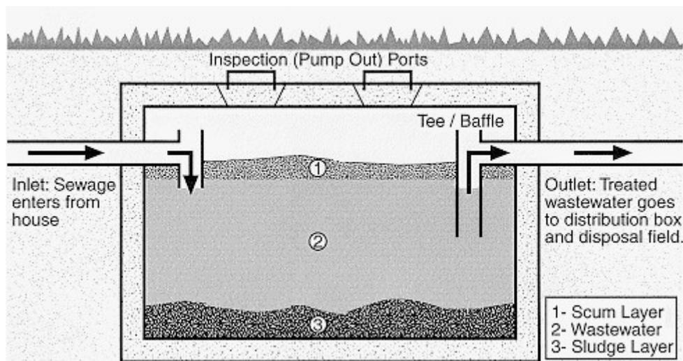
When waste enters the tank, bacteria begin to break down the solid materials. This break down reduces solids, but also leaves a residue
