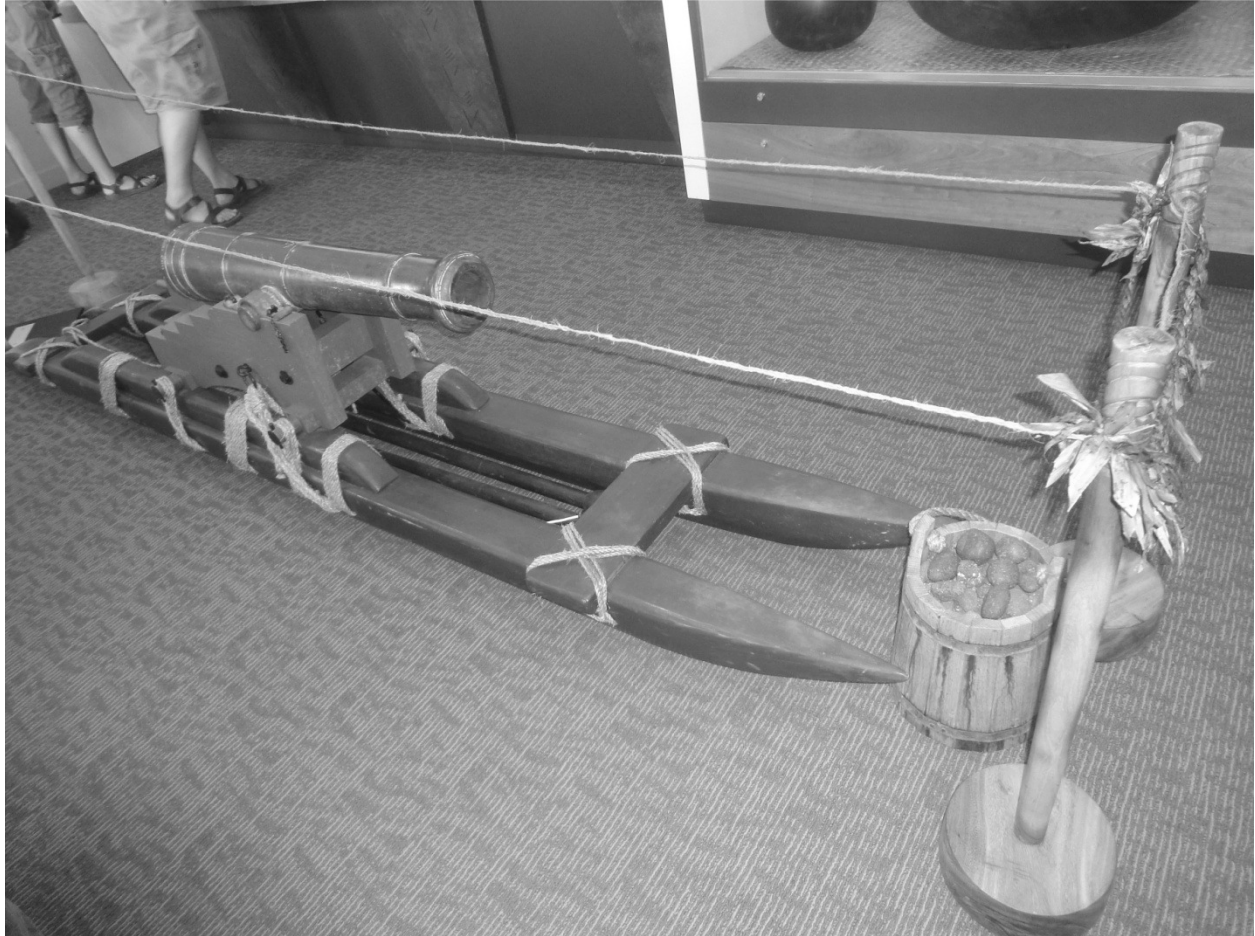
Fig. 2. Foreign weapons, such as cannon, were adapted for use in Hawaii. This weapon, from the Pu'ukohola Heiau National Historic Site, Hawaiian Island, is mounted on wooden skis to make it easy to move over the lava and hillsides. It also shoots rocks, such as those in the basket to the right, rather than cannon balls. Photo by author.
