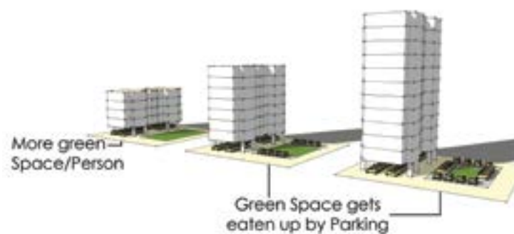
Figure 7. Effect of increasing FSI on soft ground
