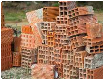
Figure 150: Stack of Hollow Clay Blocks with Horizontal Perforation Source: Adobe Stock Image
