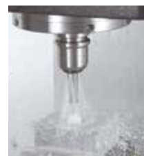
CCK collet & CKFN nut The Jet Coolant Pressure creates a tornado effect, ensuring efficient swarf dispersal.
