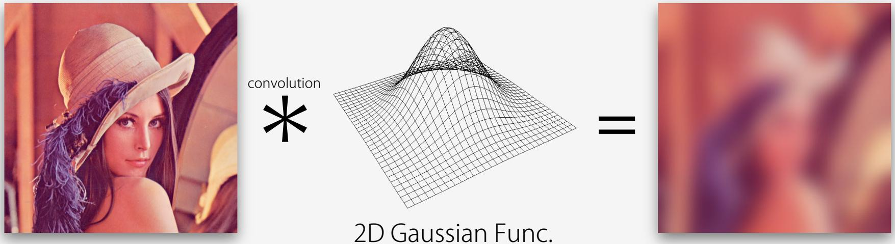
**Figure** Image Blurred by 2D Gaussian Filter
