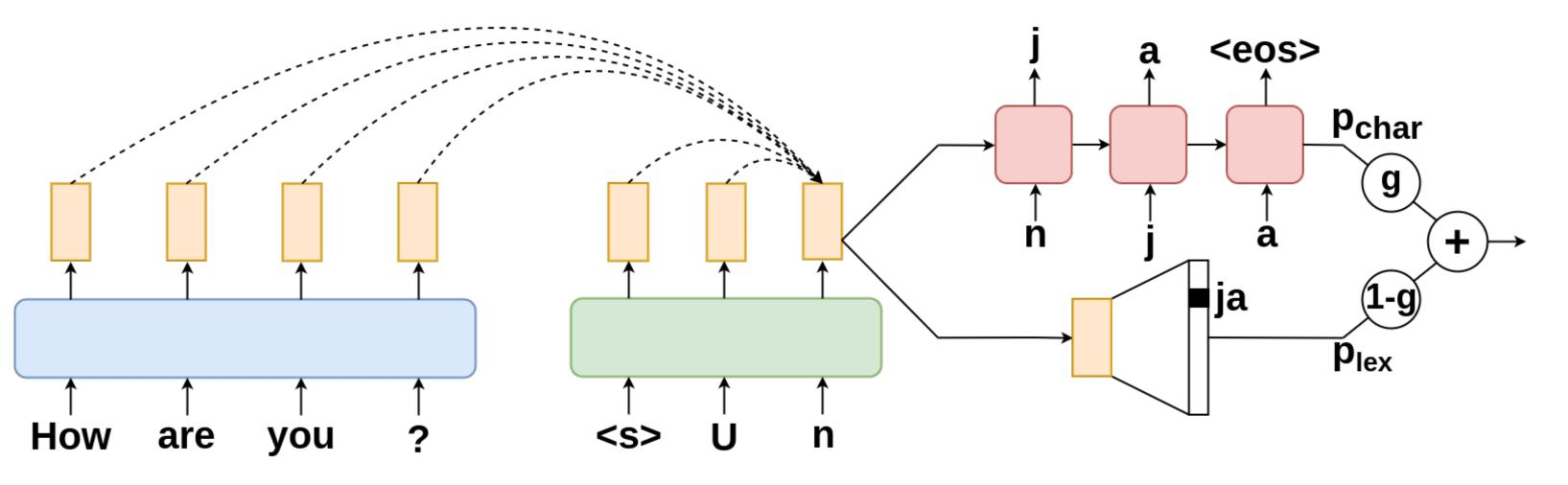
SSMT translates "How are you?" to the Zulu "Unjani?", computing the probability for subword "ja". A Transformer encoder-decoder encodes the BPE-segmented source sentence and character-level target sentence. A mixture between a character decoder and lexicon model produces the next subword probability:  $\begin{array}{ll} + \text{lexicon} - \text{char} (\text{SSMT} - \text{char}) & 26.2 \\ + \text{lexicon} + \text{char} (\text{SSMT}) & \mathbf{26.4} \end{array}$
