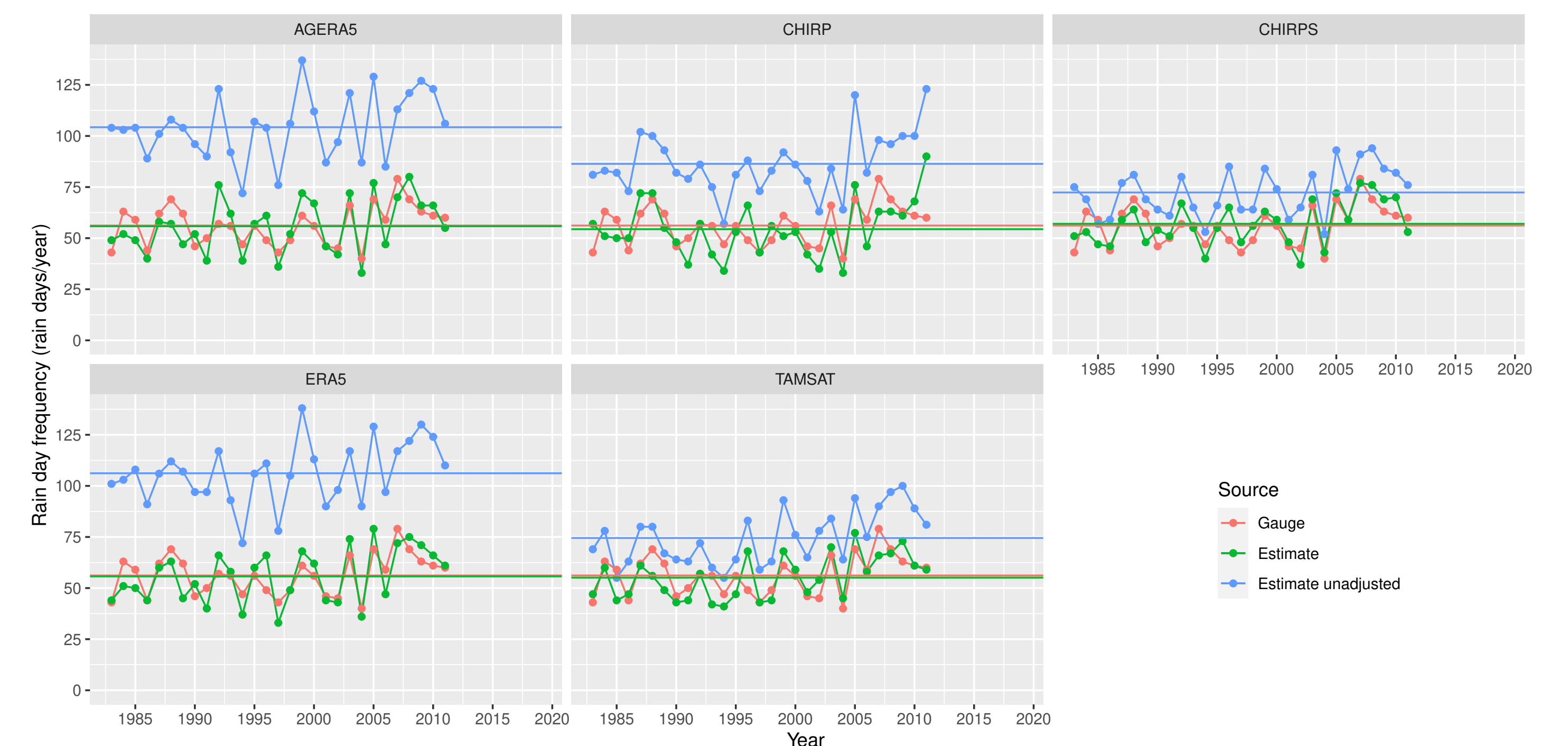
Figure 4. Gauge vs product estimates vs bias-corrected estimates - rain day frequency (rain days/year)
