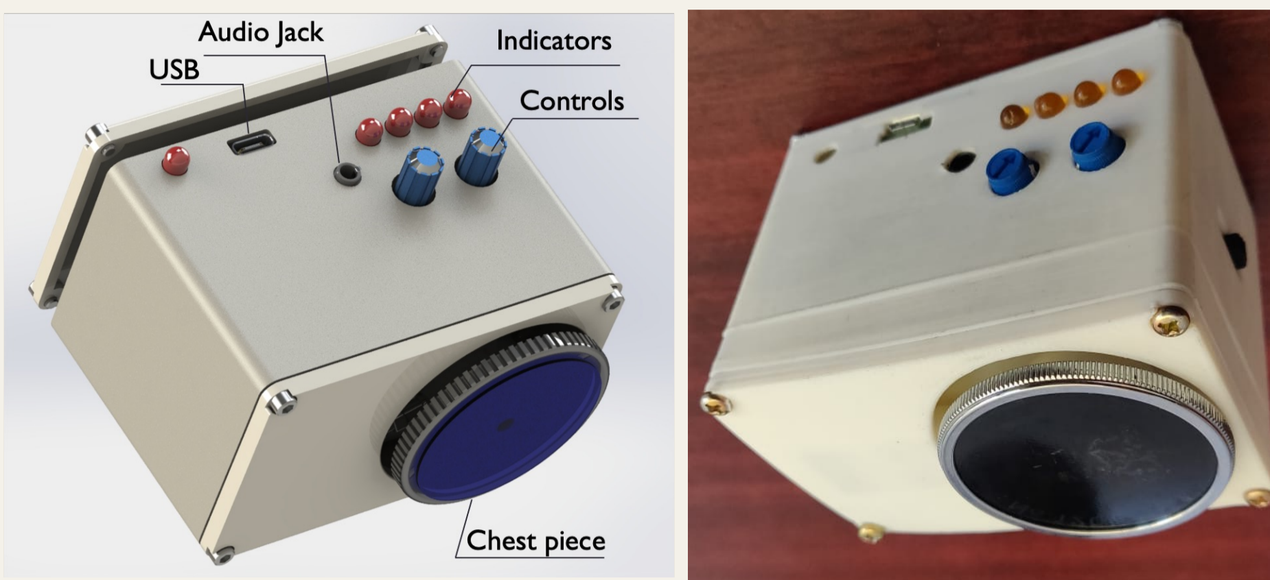
Digital Stethoscope CAD model & Prototype
