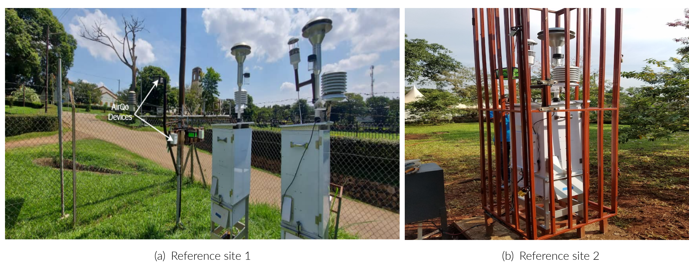
Figure 1. Monitoring sites used in this study. Part (a), shows AirQo devices and BAMs installed at Makerere University (Reference site 1), part (b), shows AirQo devices and BAM installed at Nakawa (Reference site 2)
