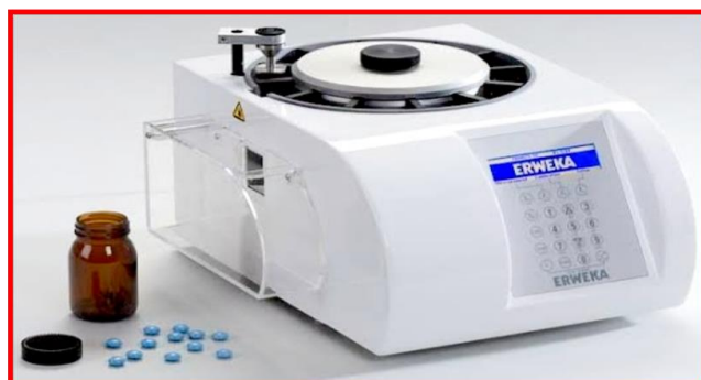
Figure 11: Erweka hardness tester.
