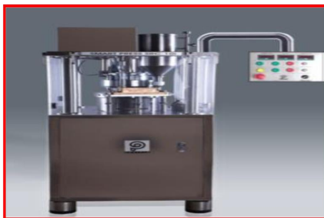
Figure 9: (c) Bilayer tablet press with displacement monitoring.
