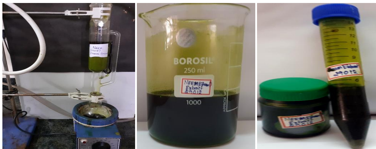
Fig. 1: Soxhlet extraction and neem extract.
