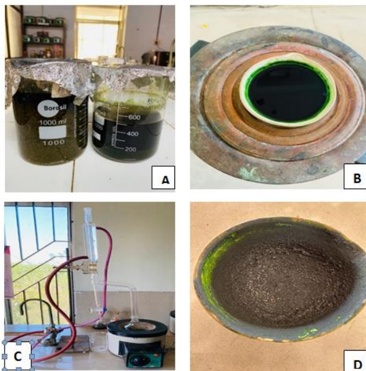
Fig. No. 4: A-Maceration; B-extract; C-distillation unit, D-dried extract.
