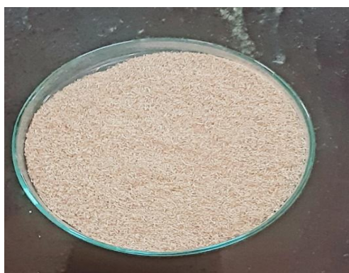
Fig. 3: The Nanocellulose particles of the plant Alangium salviifolium .
