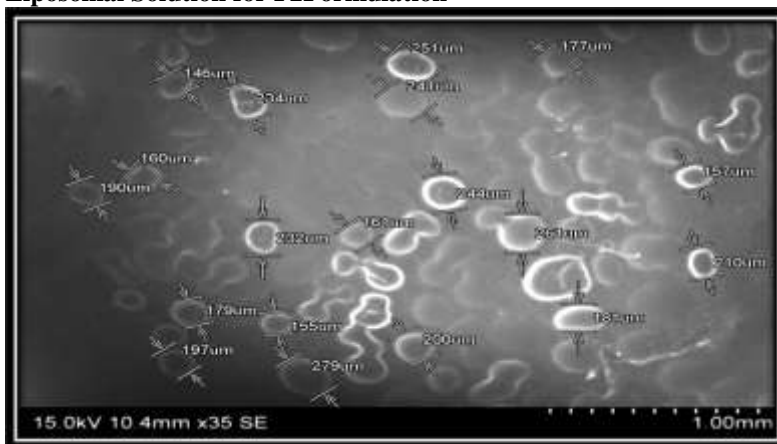
Figure 3: Figure Shows SEM Photography of Liposomal Solution for F2 Formulation.
