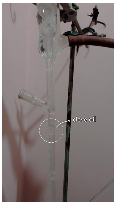
Img. 5: Accumulation of clove oil in receiver tube.
